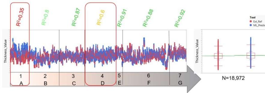
Figure 6. Comparison of thin film thickness results from external reference (Ext\_Ref) and ML model (ML\_Predict). For 18,972 sampling dies, the averaged ML predicted thickness has 0.13% higher mean, and 7.9% higher overall standard deviation than the external reference.
