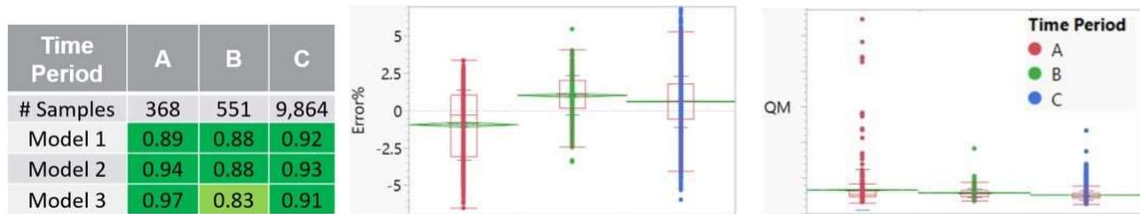
Figure 13. R<sup>2</sup> matrix, Error % and QM blind test trend for BEOL E-test Prediction model.
