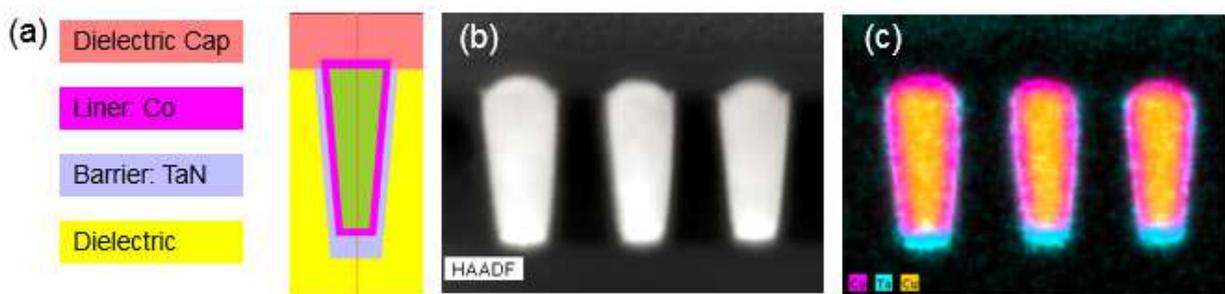
Figure 7 shows the cross-sectional structure of Cu metal lines. (a) shows the schematics of the structure. (b) shows the high-angle annular dark-field TEM image, from which the metal and dielectric are clearly distinguished. (c) shows the elemental mapping image from EDX-TEM measurement, where the TaN barrier, Co liner and Cu are clearly resolved.
