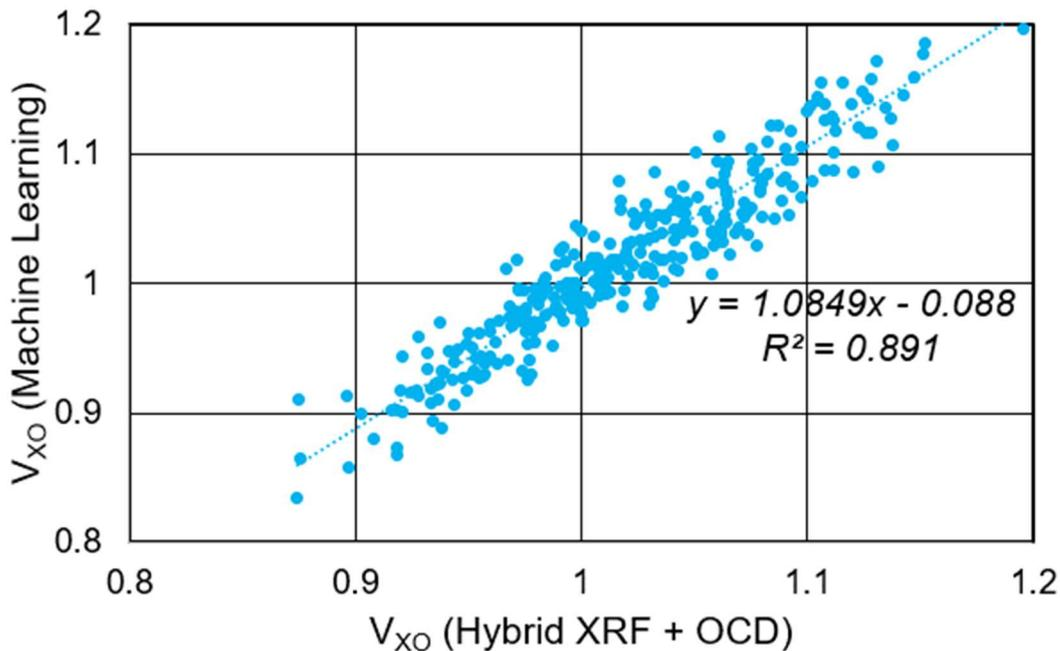
Figure 15: Comparing machine learning and hybrid results. The machine learning method is employed to predict  $V_{xo}$  based only on scatterometry raw spectra. The actual measured  $V_{xo}$  is used as reference for machine learning algorithm setup with respect to scatterometry raw spectra. The predicted  $V_{xo}$  from machine learning highly correlates with the actual measured  $V_{xo}$  from hybrid metrologies.
