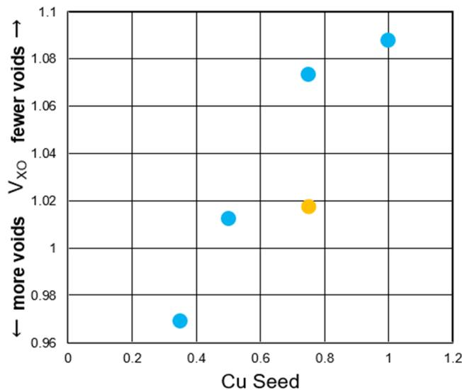
Figure 12: The metric of  $V_{xo}$  is plotted against Cu seed layer thickness. The blue datapoints are wafer averages for no reflow splits, and the yellow datapoint is that with reflow split. Blue datapoints shows a strong correlation between  $V_{xo}$  and Cu seed thickness. This relationship matches the expectation from process knowledge.
