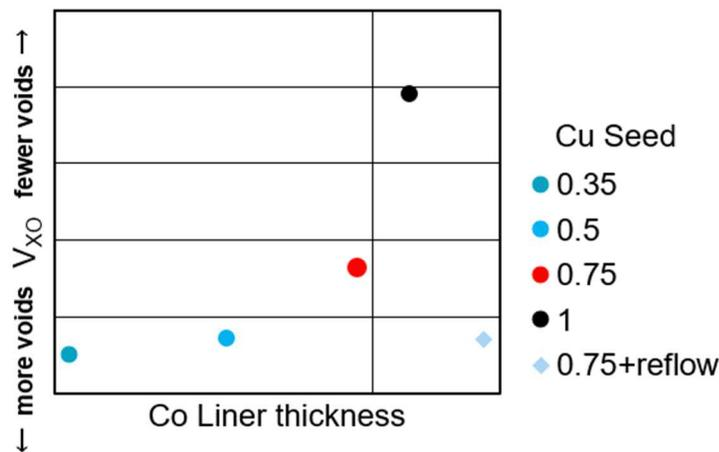
Figure 13:  $V_{xo}$  as a function of Co Liner Thickness. The metric of  $V_{xo}$  is plotted against Co liner thickness in terms of wafer average. The circular data points are from no reflow splits, and the diamond data point is from with reflow splits. The circular data points follows nice trend versus Co liner thickness, which agrees with expectation from process point view. The no-reflow data point flies away the trend.
