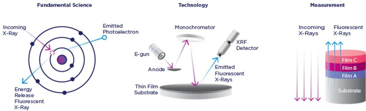
Figure 4: Schematic of low energy x-ray fluorescence measurements
