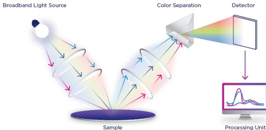
Figure 3: Schematic of optical scatterometry measurements.
