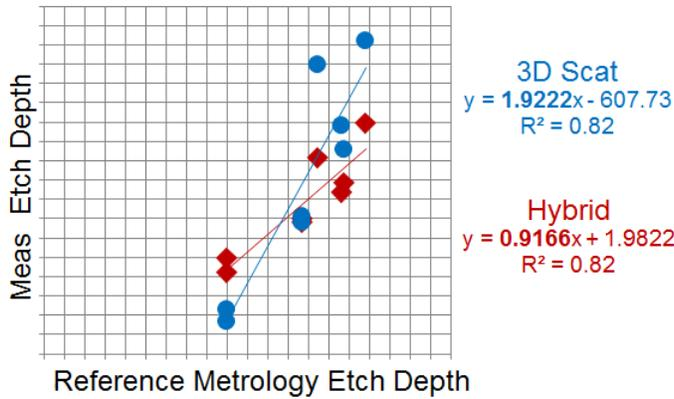
Figure 8: Correlation of hybrid scatterometry and 3D scatterometry ILD etch depth to reference metrology.
