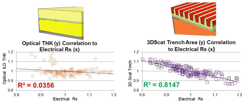
Figure 1: Comparison of correlation of 1D optical measurement and 3D scatterometry measurement to electrical resistance parameter [1]
