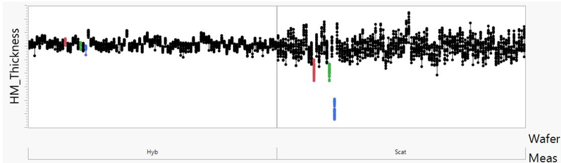
Figure 4: Comparison of hybrid scatterometry and 3D scatterometry hard mask thickness for 14nm wafers.
