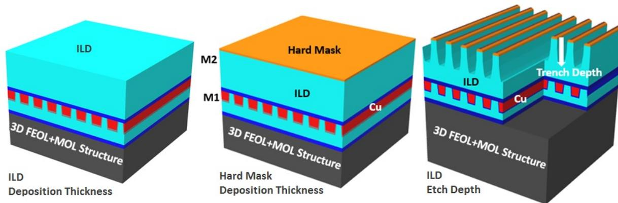
Figure 2: Schematic of measurement structure used for interlayer dielectric (ILD) thickness, hard mask thickness and interlayer dielectric trench depth measurements.
