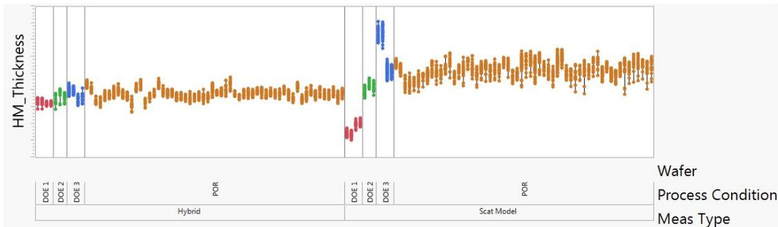
Figure 5: Comparison of hybrid scatterometry and 3D scatterometry hard mask thickness for 14nm wafers including incoming process DoE conditions.
