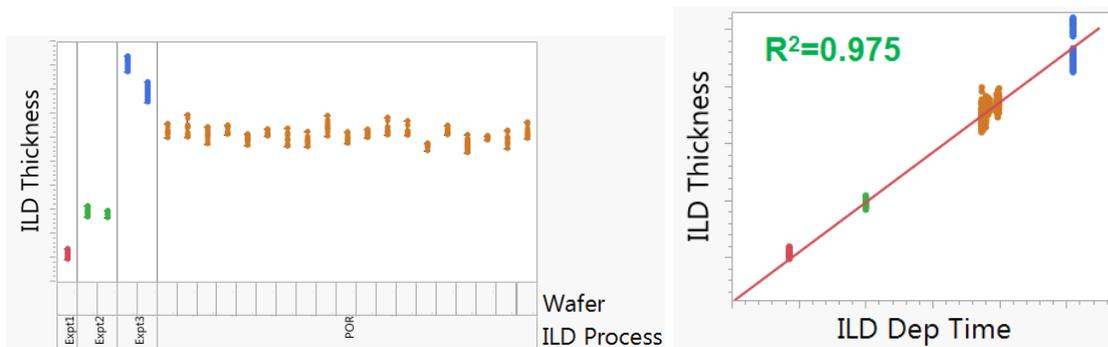
Figure 9: Measurement of ILD thickness by ILD process grouping and correlation of ILD thickness to ILD dep time
