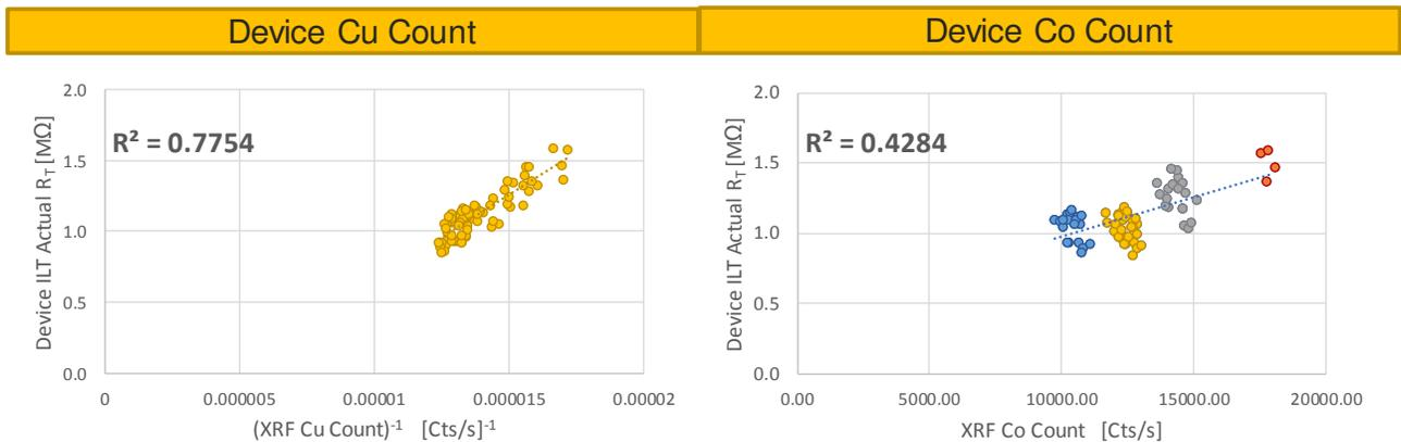
**Figure 7:** Comparing XRF data to measured resistance. For the Co count, the different Co liner thickness splits are shown in different colors. The presence of a nominally-constant Co cap on top of the Cu line is adding some noise to the Co measurement, likely reducing the quality of the correlation.
