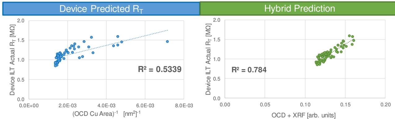
**Figure 8:** Hybrid Predicted Resistance (on right) compared to ILT. On the left are the results without the use of XRF. In both sets of data, the same die and the same measurement target (device) were used.
