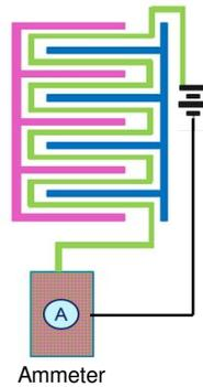
**Figure 1:** Schematic of device test structure.
