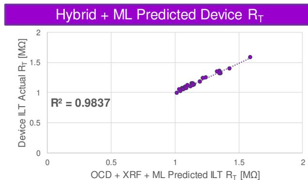
**Figure 9:** Hybrid + Machine Learning Predicted Resistance compared to ILT. The same sampling was used here as was used for the data in figure 8.
