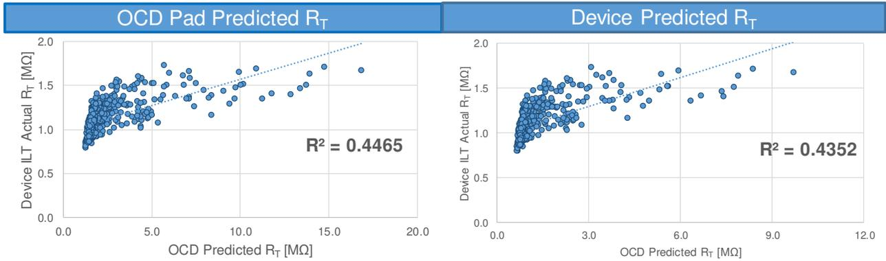
**Figure 6:** Calculating resistance based on OCD’s measured cross sectional area of Co liner and Cu and comparing to measured resistance.
