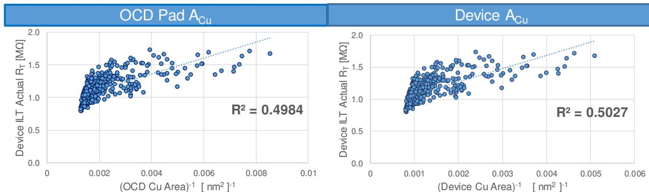
Figure 5: Comparing cross-sectional area of Cu to measured resistance.
