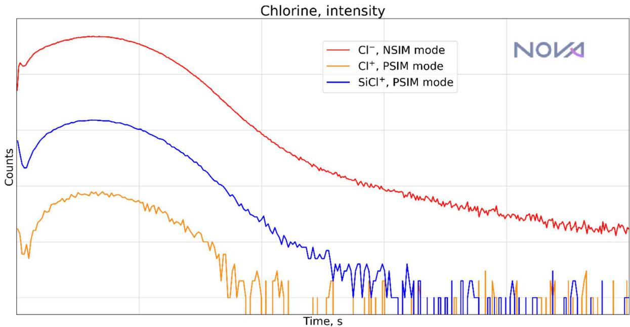
Figure 3. Comparison of sensitivity to Chlorine and SiCl<sup>+</sup> as proxy to Chlorine in negative and positive ion modes.
