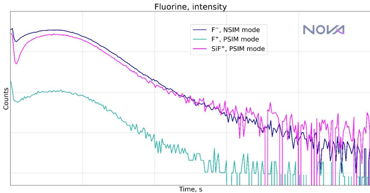
Figure 6. Comparison of sensitivity to Fluorine and SiF<sup>+</sup> as proxy to Fluorine in negative and positive ion modes.
