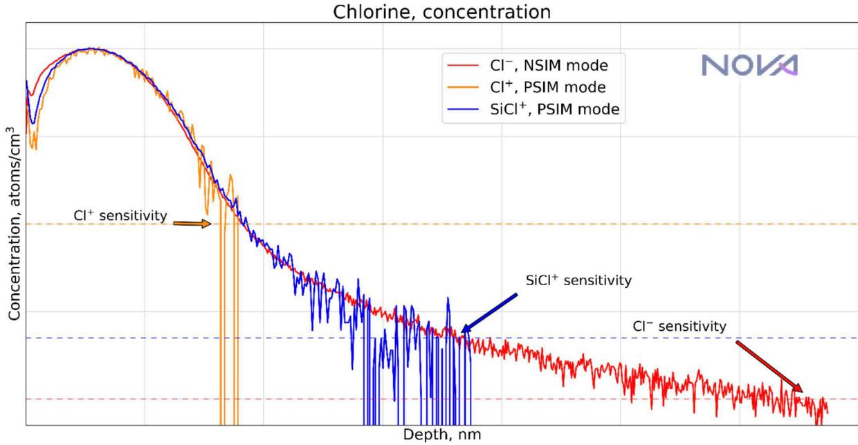
Figure 2. Chlorine implant in Silicon profile of concentration (atoms/cm<sup>3</sup>) as a function of depth (nm). Measurements in PSIM and NSIM mode provide consistent information, including proxy species of SiCl<sup>+</sup>.
