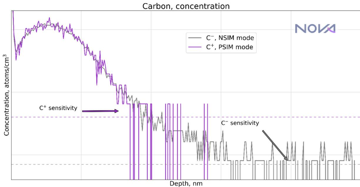
Figure 7. Carbon implant in Silicon profile of concentration (atoms/cm<sup>3</sup>) as a function of depth (nm). Measurements in PSIM and NSIM mode provide consistent information.
