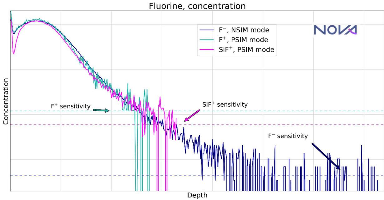
Figure 5. Fluorine implant in Silicon profile of concentration (atoms/cm<sup>3</sup>) as a function of depth (nm). Measurements in PSIM and NSIM mode provide consistent information, including proxy species of SiF<sup>+</sup>.
