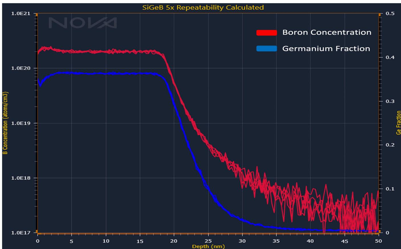
Figure 3. Repeatability of B concentration and Ge fraction measured in B doped SiGe epitaxy with METRION® at 500eV primary beam energy.
