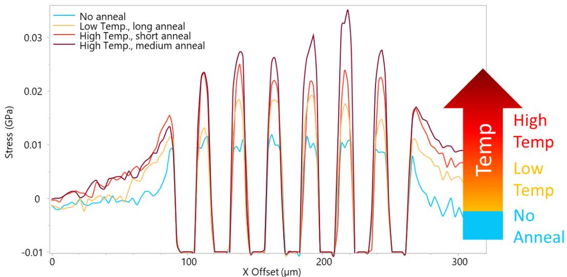
Fig. 8 Stress distribution for line scans over the same 26  $\mu\text{m}$  pitch TSV array on different wafers exposed to a variety of annealing conditions ranging from no anneal to high-temperature annealing. Note, for the high temperature annealing step, two different durations were considered indicated by lighter and darker shaded of red.
