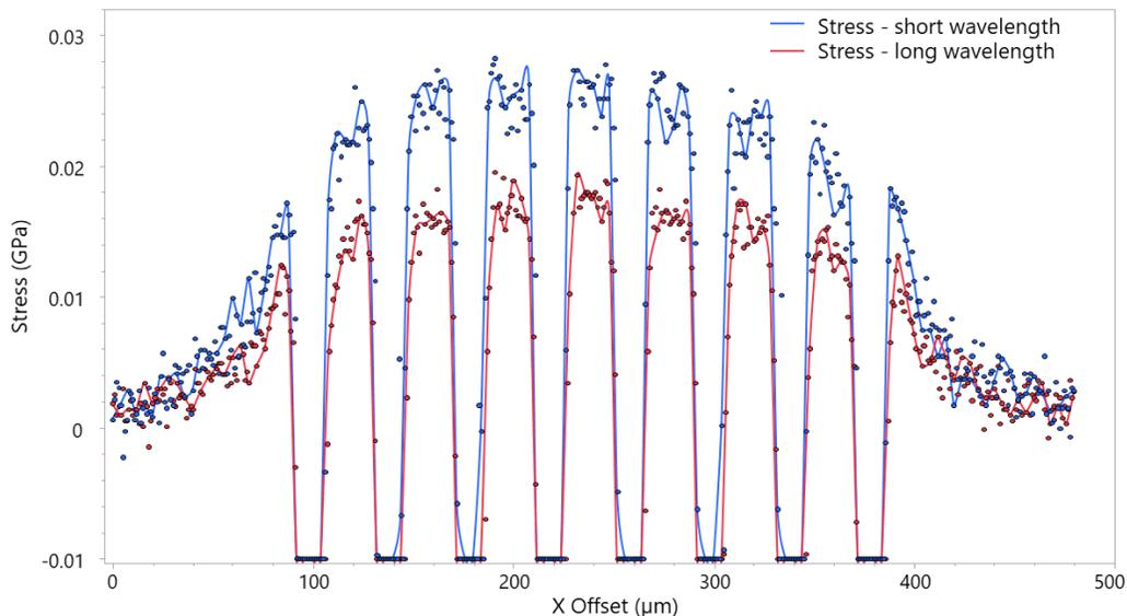
Fig. 10 Stress distribution for a 26  $\mu\text{m}$  pitch TSV array obtained on the same wafer using two different excitation laser wavelengths. The longer wavelength laser light penetrates deeper into the Si substrates and thus probes stress at deeper levels than the short wavelength laser light.
