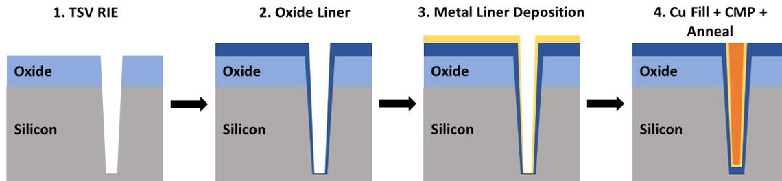
Fig. 1 Sequence of TSV processing consisting of TSV RIE, oxide liner deposition, metal liner deposition, Cu fill, overburden CMP, and an annealing step.
