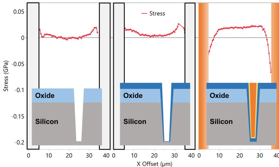
Fig. 4 Stress evolution for line scans between the same two TSVs in a 40  $\mu\text{m}$  pitch array for wafers measured after different processing steps as indicated by the sketches in each column. The position of the TSVs is indicated by the columns at  $x = 0 \mu\text{m}$  and  $x = 40 \mu\text{m}$ , respectively.
