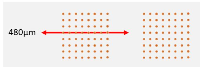
Fig. 2 Example of a line scan for the  $40 \mu\text{m}$  pitch arrays. Dots indicate the position of the TSVs and the arrow symbolizes the scan direction for a  $480 \mu\text{m}$  long line scan with measurement points spaced by  $1 \mu\text{m}$ .
