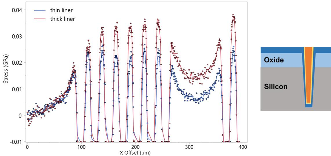
Fig. 9 Stress distribution for line scans over the same 26  $\mu\text{m}$  pitch TSV array for two different seed metal liner thicknesses (indicated in yellow in the sketch on the right).
