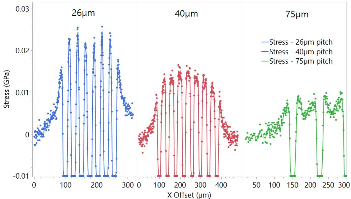
Fig. 6 Comparison of the stress distribution for line scans over square arrays of TSVs with 26  $\mu\text{m}$ , 40  $\mu\text{m}$ , and 75  $\mu\text{m}$  pitch.
