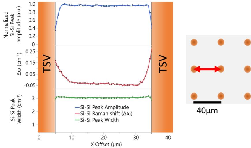
Fig. 3 Extracted peak parameters for the Si-Si bond for a line scan between two TSVs in a 40  $\mu\text{m}$  pitch array as indicated in the sketch on the right. The normalized peak amplitude, Raman shift  $\Delta\omega$  relative to the unstrained position, and the peak width are shown for the line scan between two vias of 40  $\mu\text{m}$  pitch shown in the sketch on the right.
