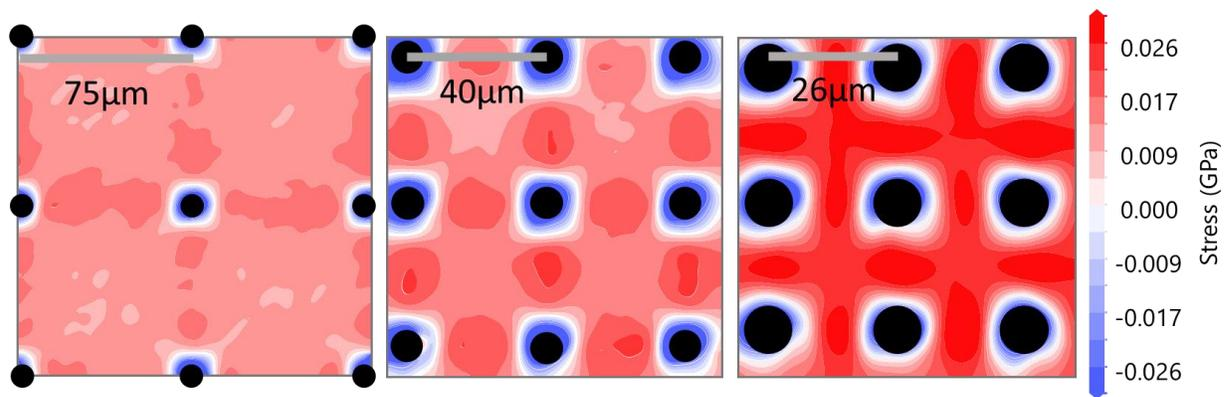
Fig. 7 Stress distribution for square maps around 9 TSVs in the center of square arrays of TSVs with 75  $\mu\text{m}$ , 40  $\mu\text{m}$ , and 26  $\mu\text{m}$  pitch, respectively. Black dots indicate the position and nominal diameter of the TSVs. All three maps use the same color scale.
