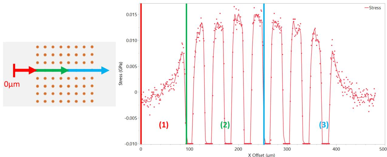
Fig. 5 Stress distribution for a line scan over a 40  $\mu\text{m}$  pitch, square array of TSVs. Three regions are identified: outside of the array and approaching the first TSV (1), between the first TSV and the center of the array (2), and from the center of the array to the opposite side of outside the array (3). Note, the expected compressive stress very close to the TSVs is truncated at -0.01 GPa, resulting in a line of data points on the x-axis marking the position of each TSV.
