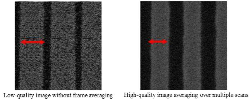
Figure 2. Example of pattern shrinkage.
