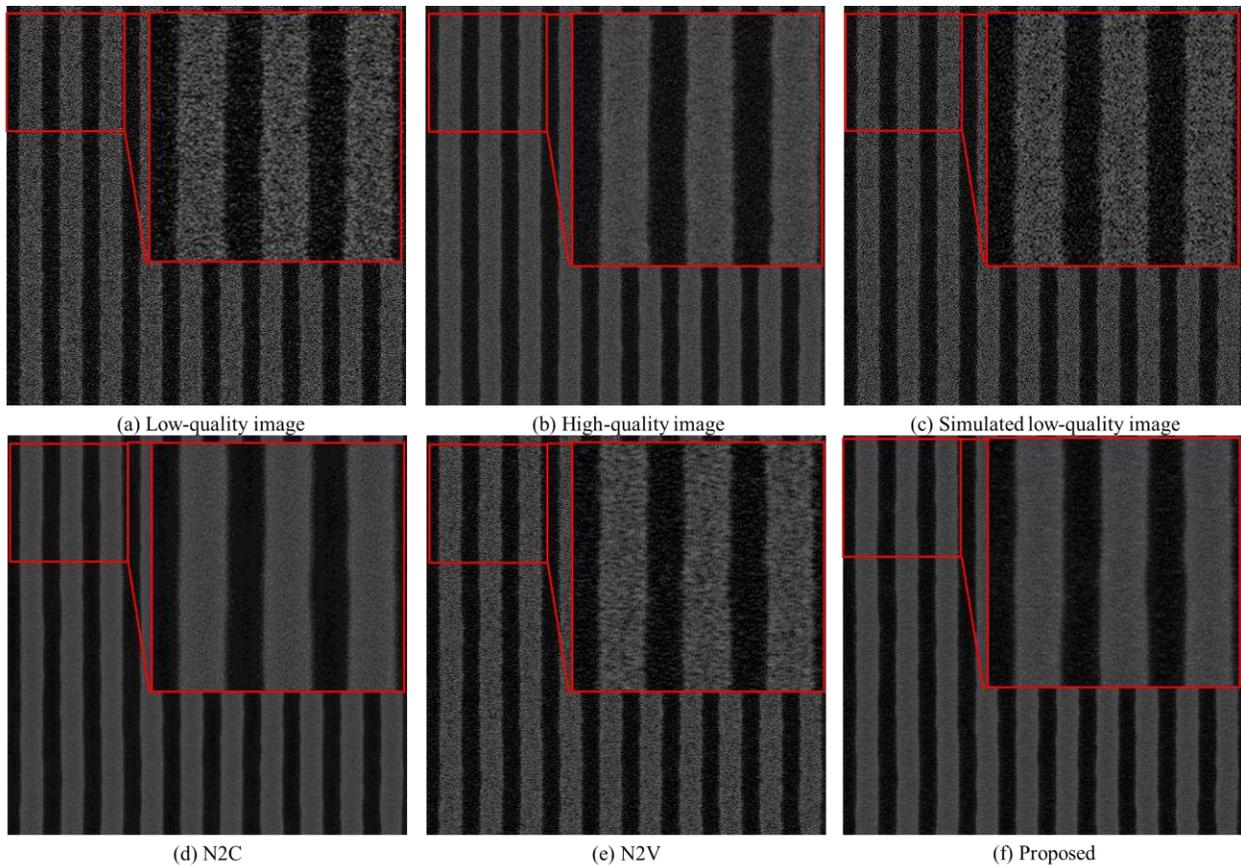
Figure 7. Examples of samples without pattern shrinkage, simulated low-quality images, and predicted results of the three methods.
