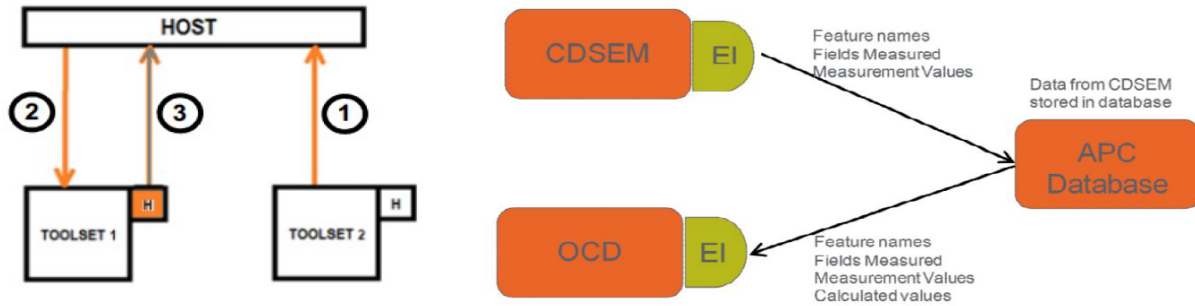
Figure 8. Left: Generic data flow between the tools and the factory system; Right: Data flow between the tools and the factory system for the “low hanging fruit” or sequential implementation [10].
